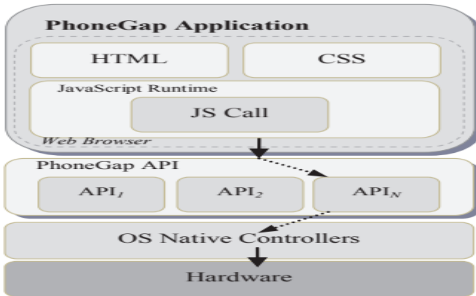
Fig. 1. PhoneGap application architecture
